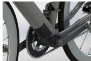
All new C19 super compact mid-motor features improved shifting performance, gear recommendation and gear indication function by GSGI sensor. – Photo COMP drives
